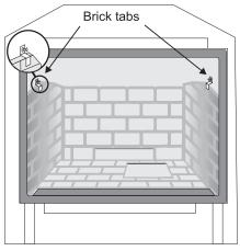
Note: If the bottom brick panel must be removed: Remove the Rear Log Stand, then remove the Burner Tray. See the "Removing Valve" section.
